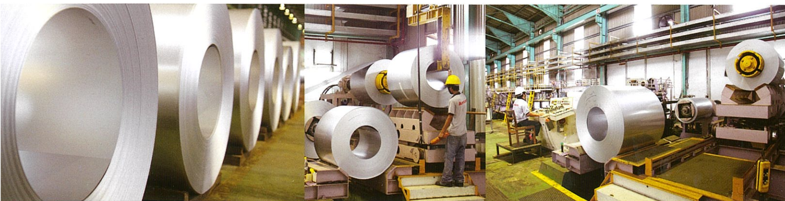
Premium 55% Al-Zn Alloy Coated Steel in Amcan Color Coating Process
