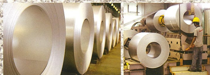
Premium 55% Al-Zn Alloy Coated Steel in Amcan Color Coating Process
